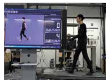
Fig. 3 Real-time motion measurement, analysis, and visualization
