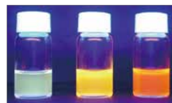
Fig. 3 Luminescence from impurity-doped semiconductor nanoparticles
