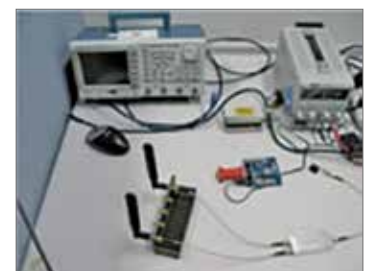
Fig. 3 ESPAR antenna assisted receiver
