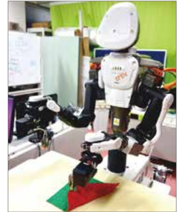
Fig. 1 Deep reinforcement learning for cloth manipulation
