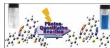
Fig. 1 Schematic illustration for photoisomerization reactions of our unique photochromic molecule, which exhibits photo-reaction with quantum yield of unity, a "photon-quantitative reaction"
