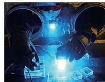
Fig. 3 Photo-irradiation process on making of organic thin-film devices
