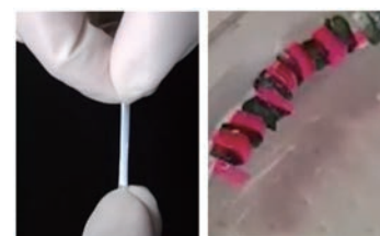
Fig. 1 Functional polyurethane based on designed monomers (left) and polystyrene oil gel.
