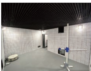
Fig. 5 Anechoic chamber for hardware security evaluation
