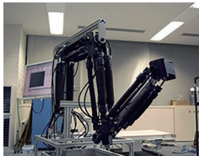
7-DOF manipulator controlled by pneumatic artificial muscles (Mathematical Informatics Lab)
