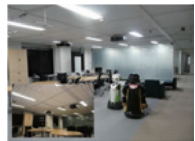
Fig.1 Experimental environments: human and robot positions are measured using laser range finders or invisible markers.
