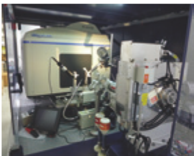
Ultra High-intensity Microfocus X-ray Generator · Macromolecular Crystallography Diffraction System
