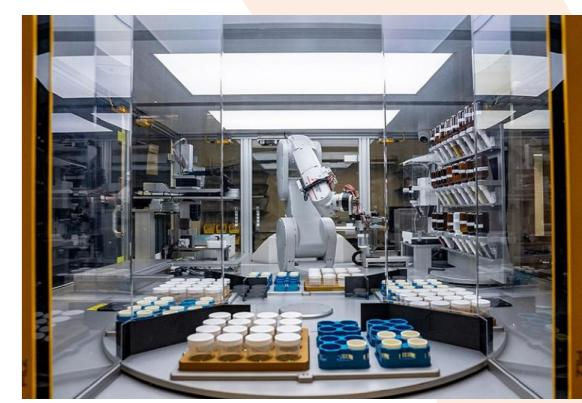
An autonomous laboratory for the accelerated synthesis of novel materials
